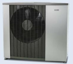
NIBE F2120 is an inverter-controlled air/water heat pump which represents a real breakthrough when it comes to efficiency. With a seasonal performance factor in excess of 5.0\*, the heat pump provides more than five times as much heat per year as an electric heater with the same energy consumption. NIBE F2120 provides optimum savings since the heat pump automatically adapts to your home's output requirements all year round.
